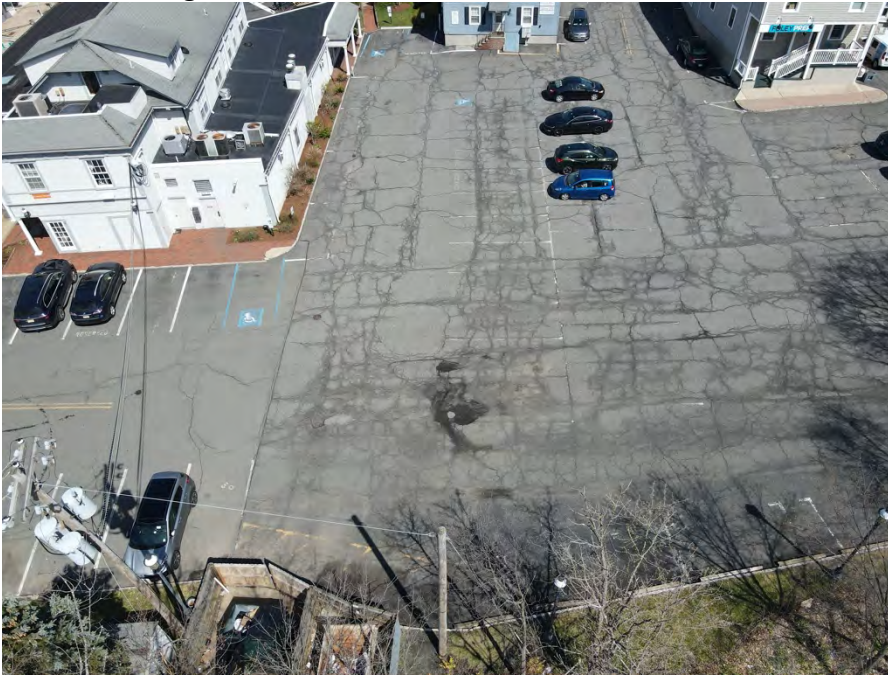
Figure 5: The directional arrows shown on the site plan are missing, which means that the intended pattern of circulation for this portion of the parking lot is not indicated. There is nothing to suggest to pedestrians or motorists that the intention is for there to be a two-way drive aisle here. Lack of directional arrows increases the likelihood of conflict.
