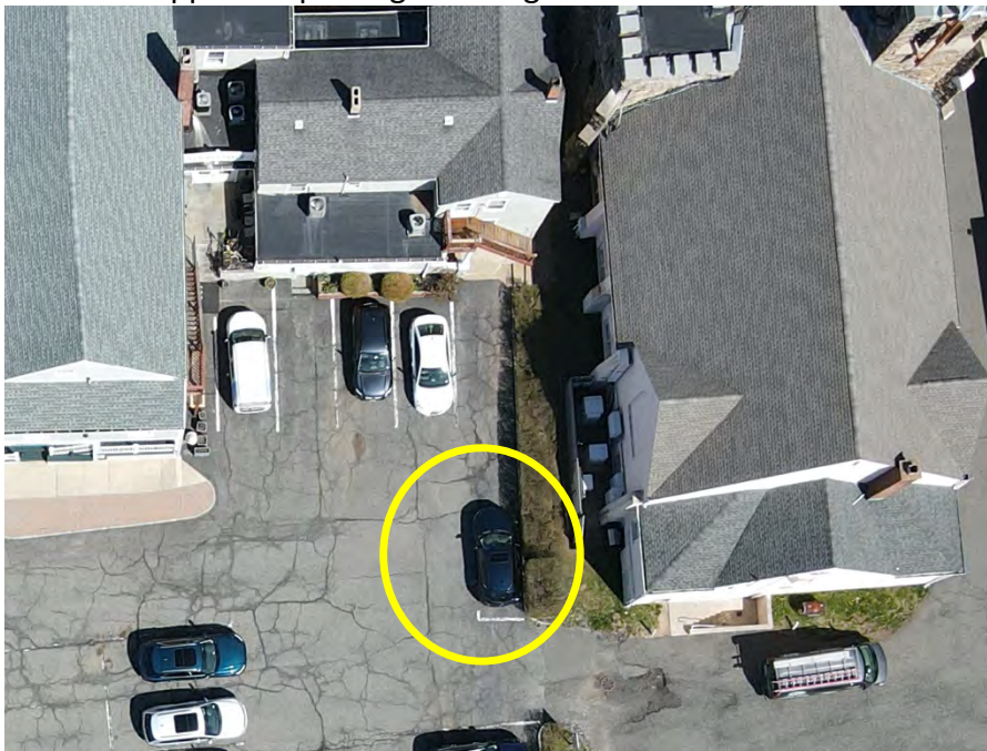
Figure 29: The parking space to the right is not shown on approved plans and serves to limit the movement of cars behind it. The arrangement also creates potential conflict points between vehicles.
