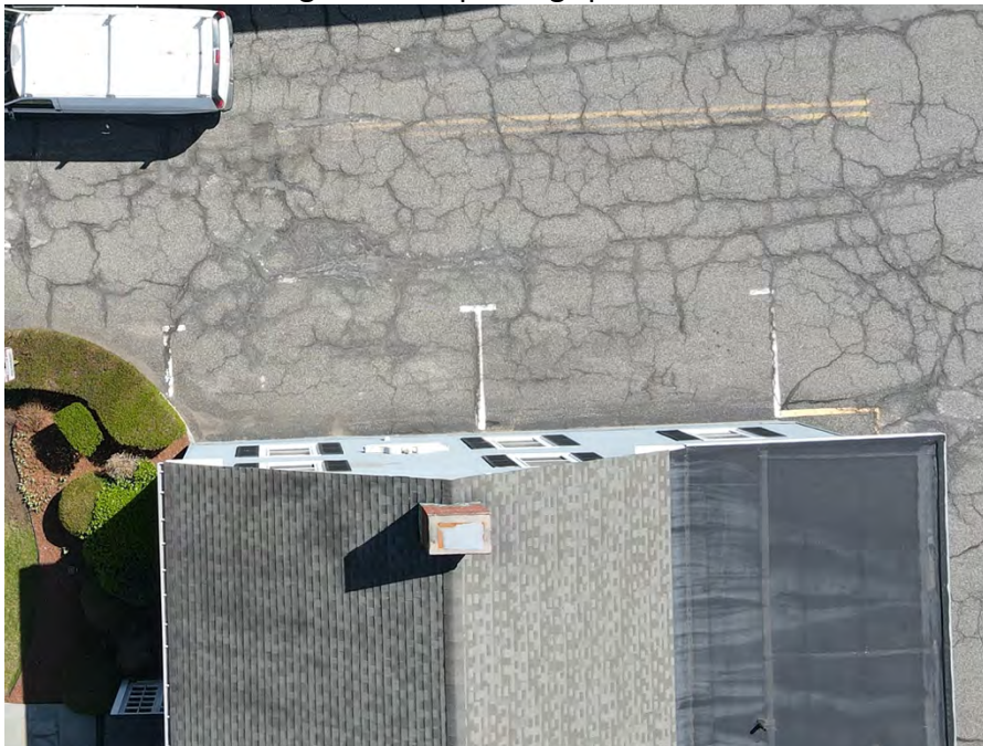
Figure 11: The site plans show a buffer here between the two parallel parking spaces on the site of 35 Olcott Square. This buffer is not present on site. Instead, the landscaping adjacent to this parking area is laid out in a manner inconsistent with the approved plan. This limits visibility for motorists entering the site from US 202, creating a blind spot conducive to dangerous conflicts between motorists and pedestrians. Faulty arrangement of this area is supported by a strip of wood along the side of the building at bumper height, which seems to have been hit repeatedly as drivers have attempted to park in this space.
