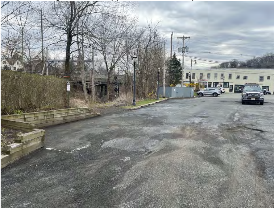
Figure 6: Unapproved parking parallel to the curb at the rear of the property. As indicated in Figure 7, the parking spaces do not meet the 9 foot minimum width requirement for parking spaces included in the Borough's Land Development Regulations.
