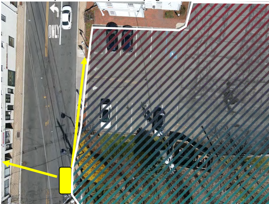
Figure 18: The entrance on the western portion of Lot 1 features a significant blind spot as motorists travelling north along Mount Airy Road have limited visibility behind a large hedge while they approach the intersection near Olcott Square along US-202.
