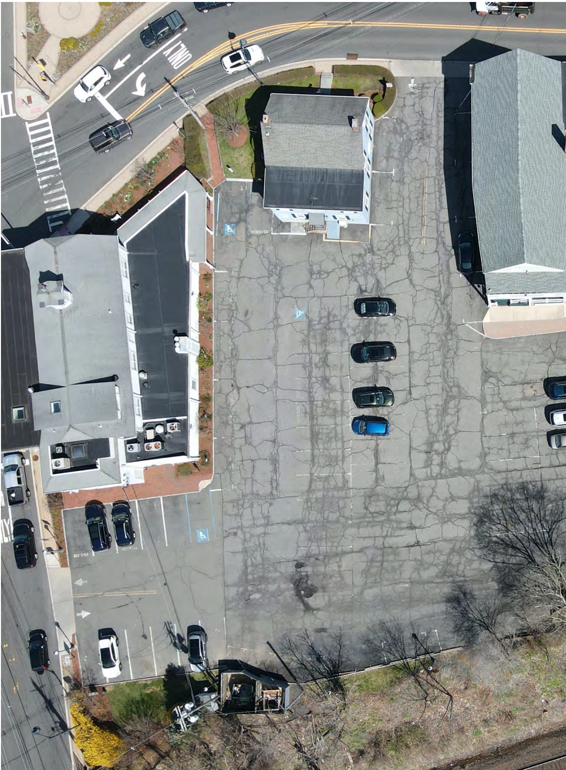
Figure 4: Aerial photograph of Lot 1 captured on April 11, 2022 showcasing faulty arrangement and discrepancies from approved site plan.
