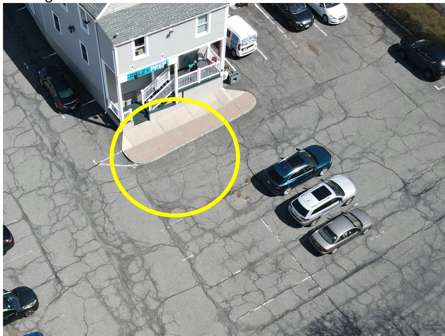
Figure 26: The site plan depicts directional arrows on the drive aisle between lots 1 and 3, which are missing. In the absence of striping, this aisle can be erroneously interpreted as a one-way, leading to motorist conflict as drivers attempt to exit or enter the lot.
