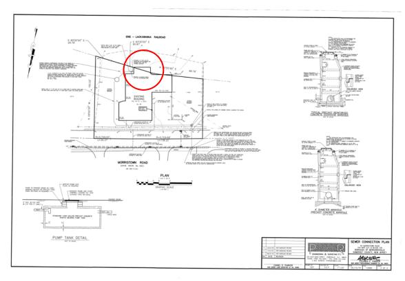
Figure 28: Sewer connection plan showing encroachment.
